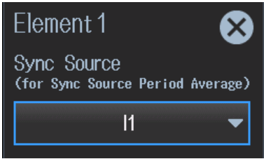
Figure 11. To change the sync source, navigate to the Setup menu and press the Sync Source button under the elements in the motor’s wiring group, then choose the proper signal from the drop-down.
