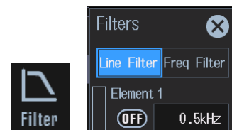
Figure 7. In the Filter menu, line filters and frequency filters for each element can be enabled and adjusted.
