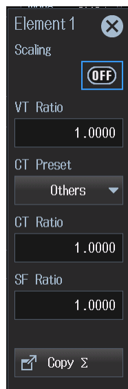
Figure 6. Users can copy the VT and CT ratios to all elements in the selected element's wiring system by pressing Copy Σ, then Copy Exec.
